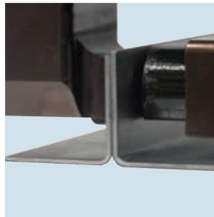
Clinchen an schmalen Flanschen Clinching on narrow flanges
