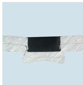
Schliffbild einer zweilagigen Clinchverbindung S-DF / Cross-section of a two-layer connection S-DF
